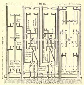
Fig. 215.—Rear elevation of the five-panel direct-current switchboard.
